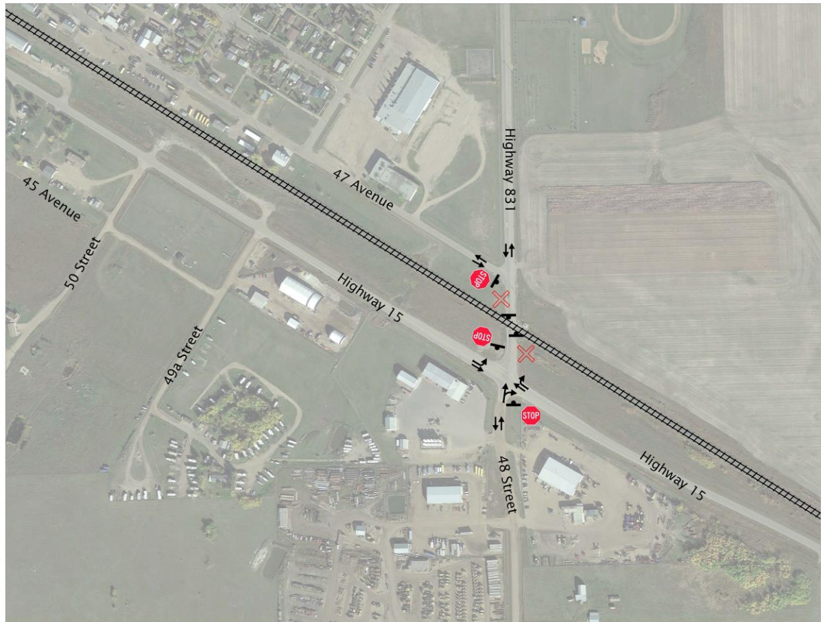
Figure 5.1 – Key features of the Hwy 831 grade crossing
